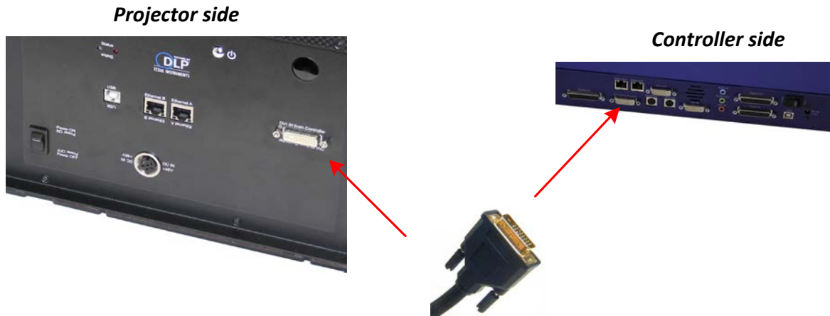
Figure 12 DVI cable between projector and controller
