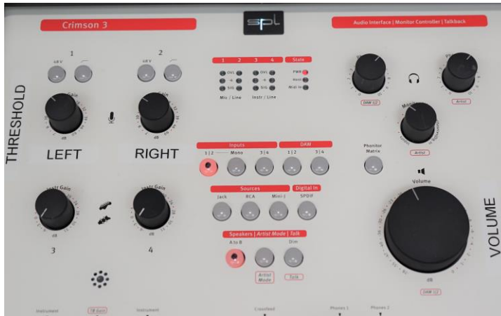
Figure 15: Crimson 3 audio volume control. The individual hearing thresholds are set using the Threshold dials on the left. Then the overall volume is increase by 60 dB by adjusting the volume dial on the right.
