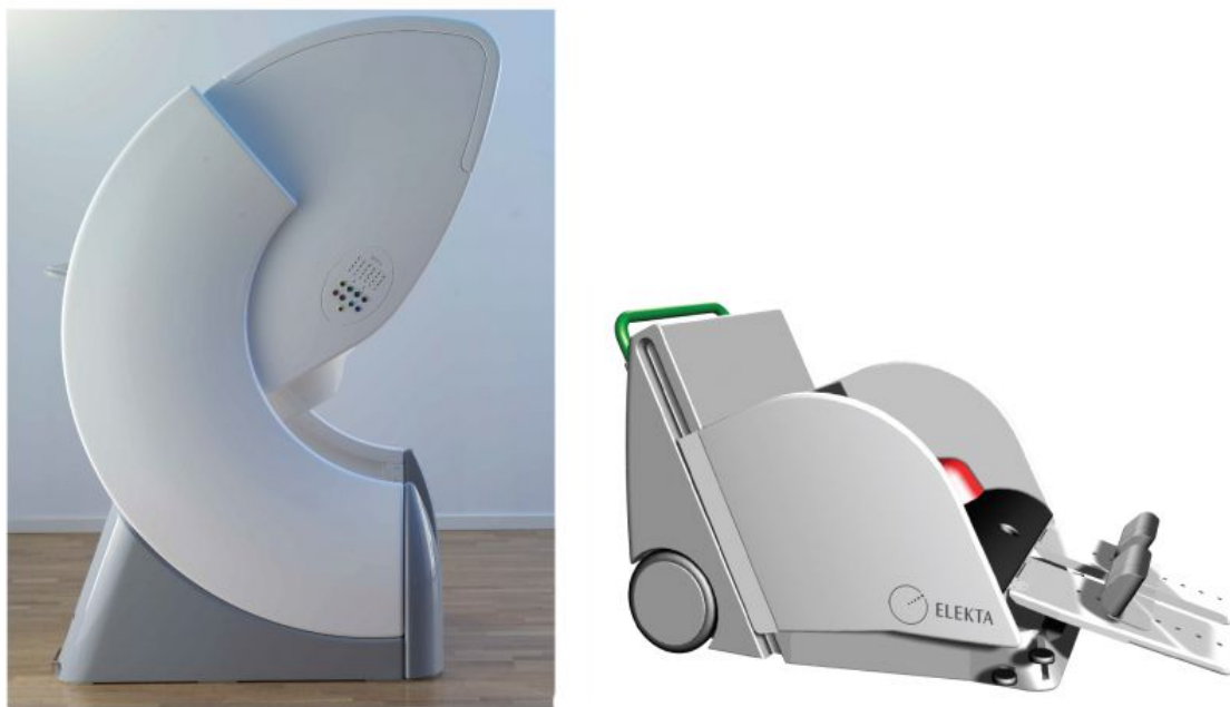
Figure 3.7 Reclined seated measurement position in the chair. The gantry tilting angle is 60° in respect to the supine position.
