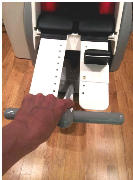
Figure 3.14 The T-bar handle installed
