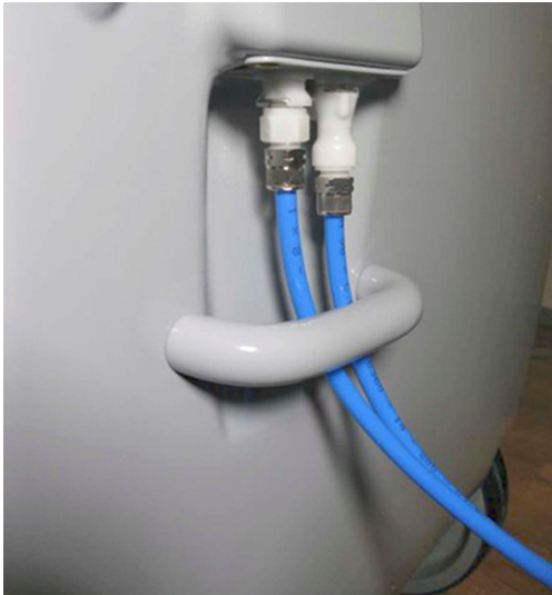
Figure 3.23 Hydraulic hoses fed under the strain relief bar and connected in the back of the chair
