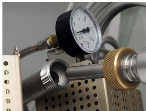
Figure 3.4 Inserting the flexible siphon into fixed siphon.
