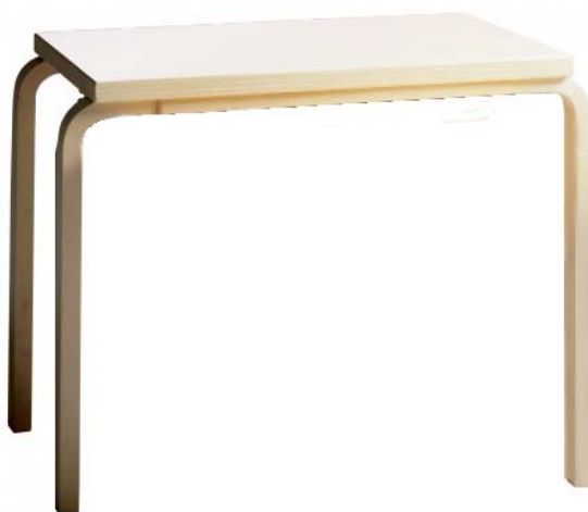
Figure 3.4 Auxiliary table for HPI coil digitization with the patient couch. The HPI coil transmitter (not shown) cable must point towards patient's feet.
