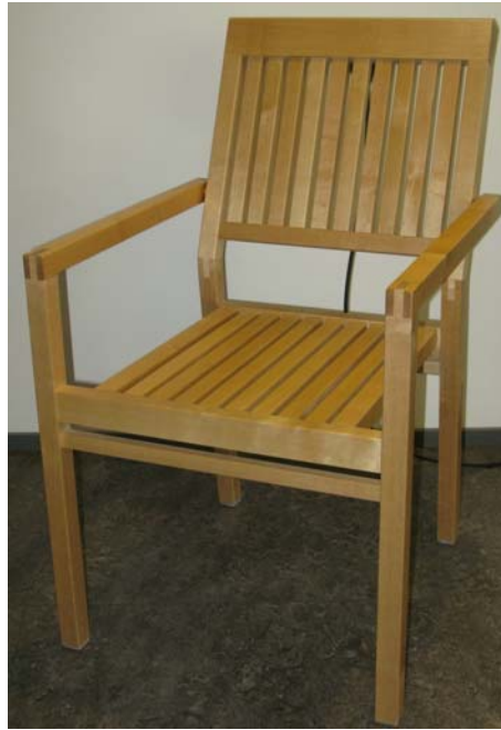
Figure 1.23 Wooden chair for digitization. Note that the transmitter coil at the back of the chair must be positioned properly to avoid problems in digitization, see section 3.3.4.
