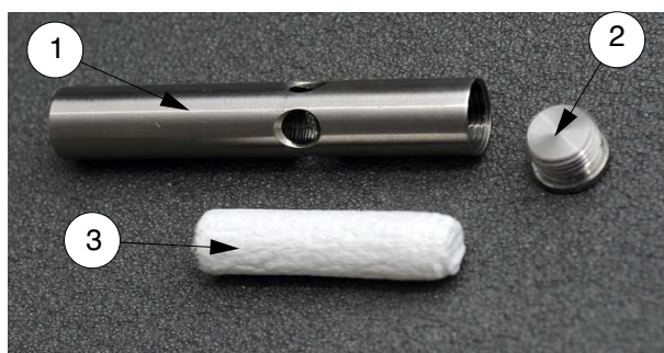
Figure 4.6 The flexible siphon filter unit. 1: Filter body, 2: end cap, 3: filter cartridge. Please note the correct orientation of the filter cartridge: the closed end must be facing towards end cap 2.
