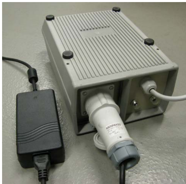
Figure 1.22 The 3-D digitizer unit power supply (left) must be connected to mains via an isolation transformer (right) supplied with the Elekta Neuromag® TRIUX.
