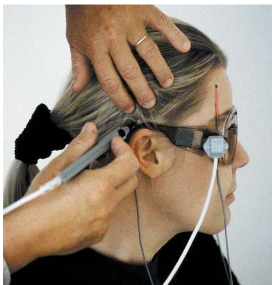
Figure 3.2 The head digitization goggles with additional receiver.
