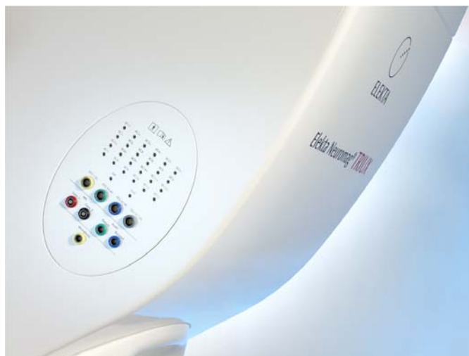
Figure 1.16 The electrode interface panel is at the probe unit side. Depending on site, it may also be located on the other side.
