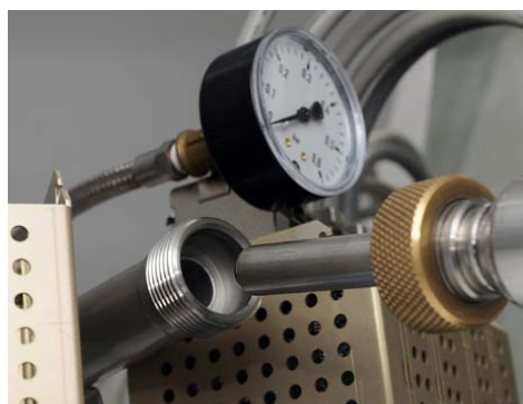
Figure 4.5 Inserting the flexible siphon into fixed siphon.
