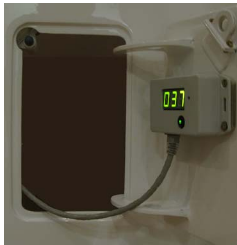
Figure 1.24 The liquid helium level display is under the hatch covering the liquid helium filling port. The liquid helium measurement can be initiated and stopped with the pushbutton.
