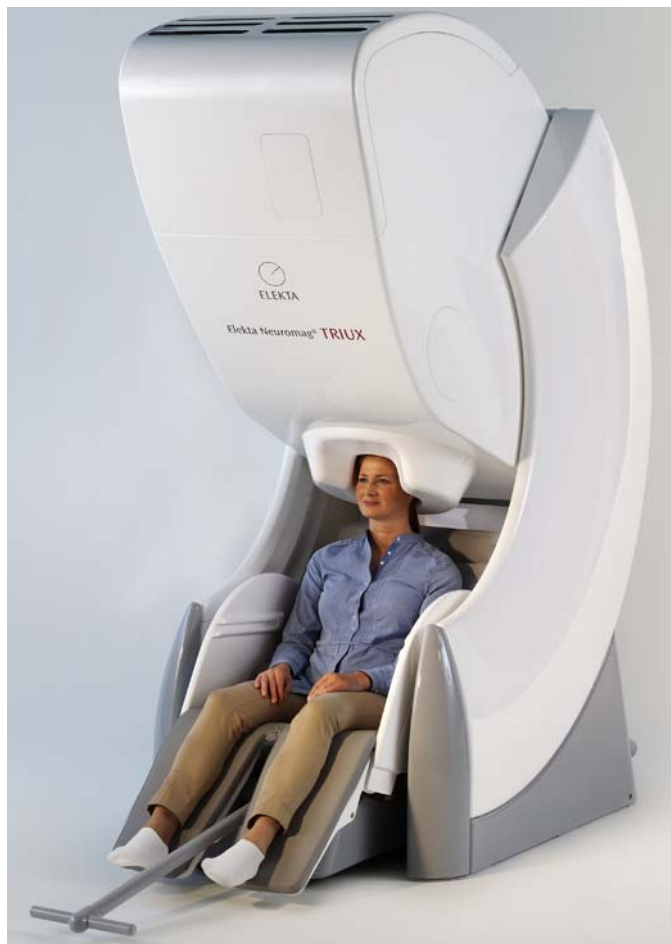
Figure 1.14 Measurement with patient seated. The probe unit has reclined and upright seated positions with slightly different tilting angles.
