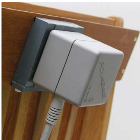
Figure 3.3 The transmitter attached to the chair. The cable must point downwards.
